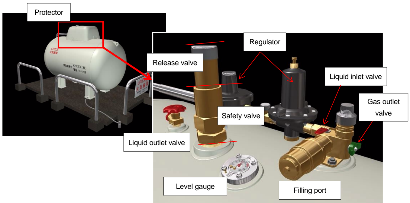
Figure 5: Bulk storage tank
