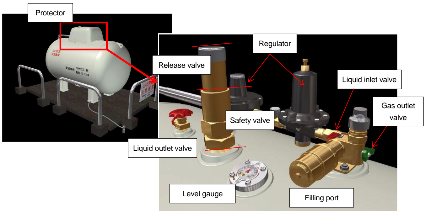
Figure 5: Bulk storage tank
