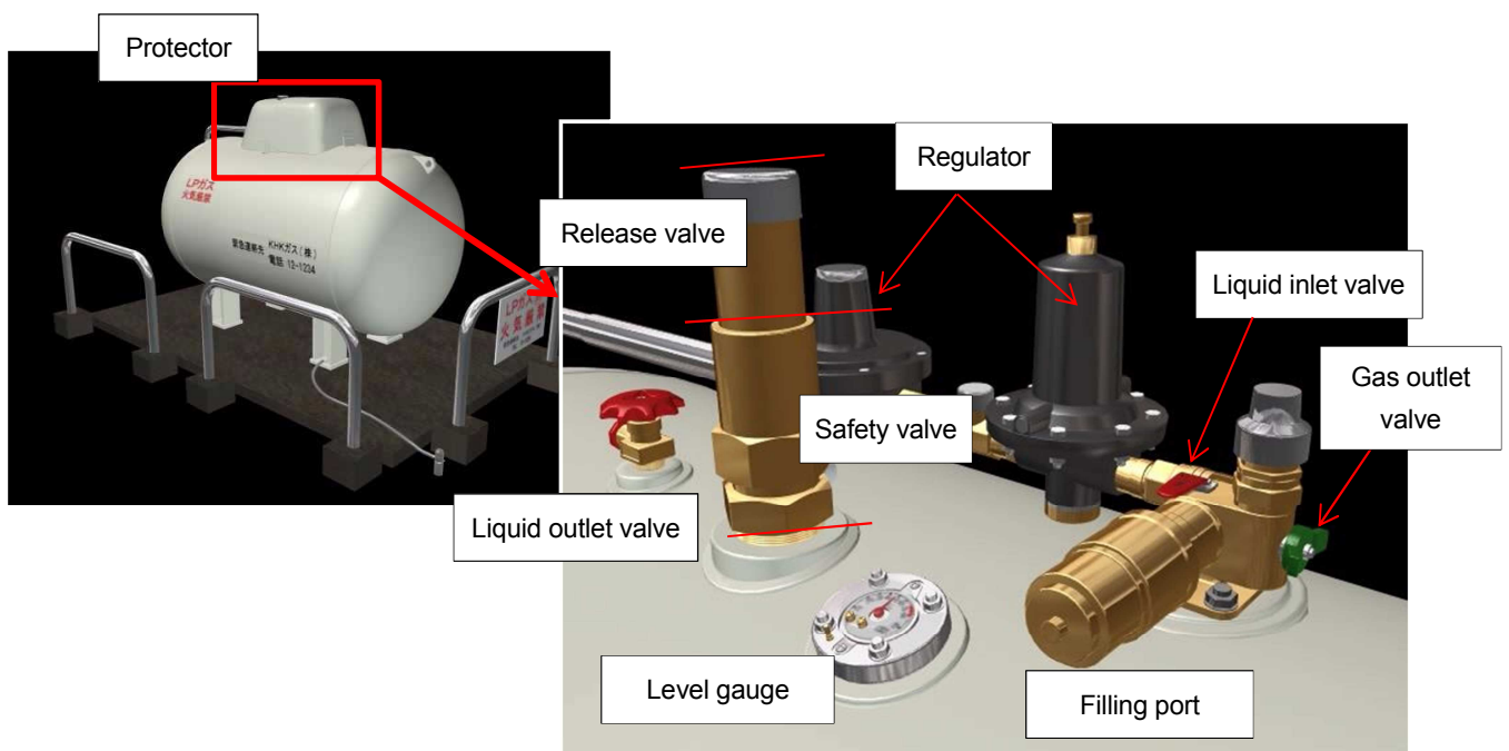
Figure 5: Bulk storage tank
