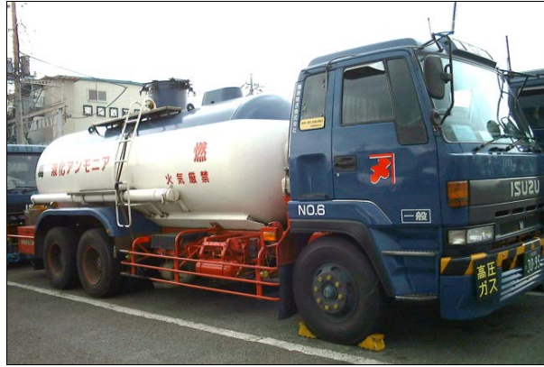
Photo 5 Transportation of liquid ammonia by a tanker truck
